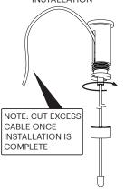
NOTE: INSTALLATION REQUIRES WIRE CUTTERS AND A STANDARD PHILLIPS HEAD SCREW DRIVER
