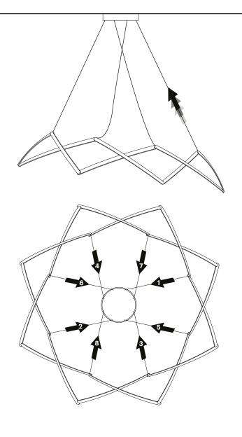
**IMPORTANT:** When raising or lowing the lamp, we recommend taking a measured approach and alternating between cables that enter the canopy opposite each other and moving around the canopy in a pattern to ensure the stress is distributed evenely accross all suspension cables. Use a long level when necessary.
