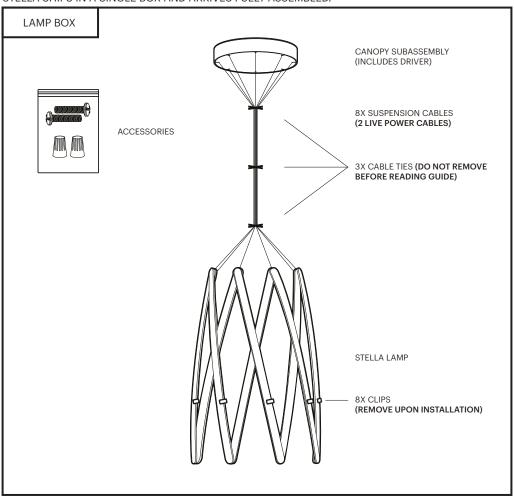
ITS CRITICAL TO AVOID TANGLING THE CABLES PRIOR TO INSTALLATION. PLEASE TAKE EXTRA CARE WHEN REMOVING THE LAMP FROM ITS PACKAGING TO KEEP THE ENTIRE ASSEMBLY IN ALIGNMENT.
