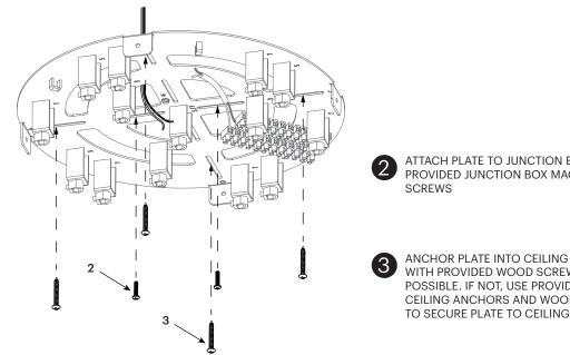
ATTACH PLATE TO JUNCTION BOX WITH PROVIDED JUNCTION BOX MACHINE SCREWS
