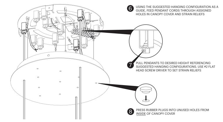
NOTE: INSTALLATION SHOWN IS FOR SOLIS CHANDELIER 3. FOR SOLIS CHANDELIER 5, FOLLOW THE SAME WIRING PROCESS USING THE HOLE PLACEMENT OUTLINED IN SUGGESTED HANGING CONFIGURATIONS
